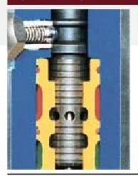
Mechanical valve eliminates expensive, unreliable electronic switching devices.
