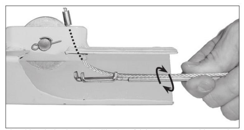
3b. With a clock-wise motion like that of tightening a screw driver, twist the cable installation tool while holding the crimped end of the cable up into the sheave pocket. The cable will pop loose from the tool and pop up through the sheave pocket as shown in this cut away view.
