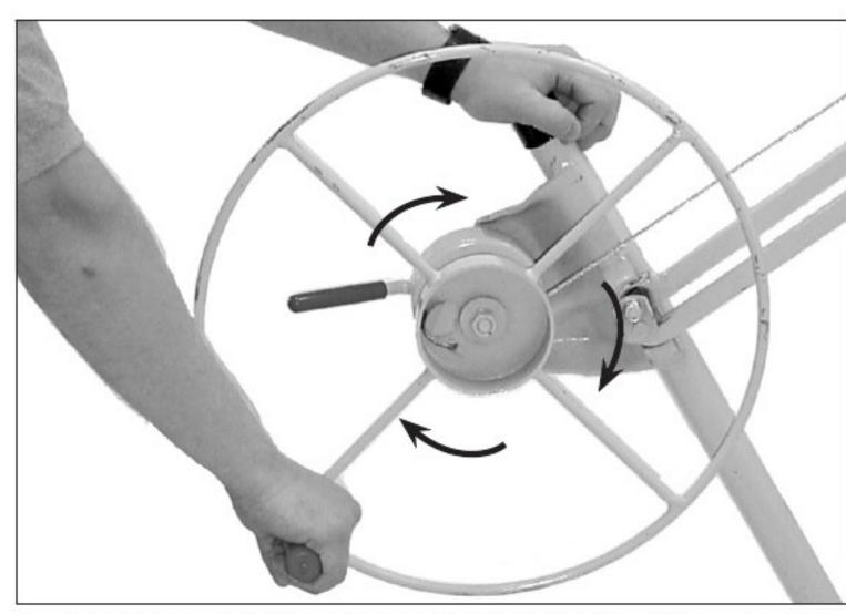
10. Rotate the winch in the direction shown to take the slack out of the cable.
