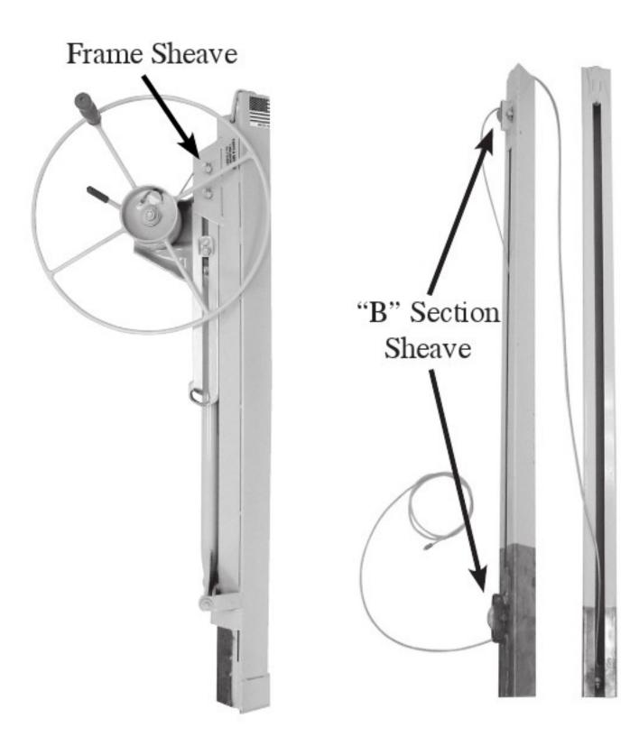
Inspect and replace sheaves (pulleys) before replacing the cable. There are 3 sheaves on the 138-2 Panellift®, one on the frame and two on the "B" telescoping section. Sheaves should be solid on their axle and not move up and down or back and forth. To replace, remove cotter keys and discard old axle and sheave. Replace with new sheave, axle and new cotter keys.
