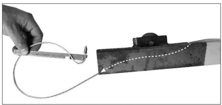
5a. Reload and insert the cable installation tool into the BOTTOM end of the "B" section as shown.
