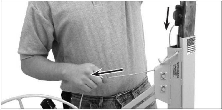
8. Pull the slack cable through the sheave pocket and slide the telescoping sections into the frame housing. As the telescoping sections lower into the frame, the slack cable will be drawn back up over the sheave.
