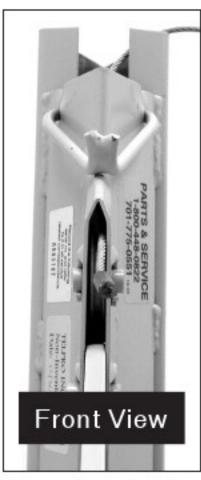
7. To reinstall the assembled telescoping sections, feed the crimped end of the cable through the frame sheave pocket from the top and over the top of the sheave as shown. (Model 182 go to page 13)
