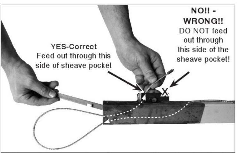
5b. Repeat the process performed in steps 2 - 3: Insert the crimped end of the cable up into the end of the sheave pocket at the end nearest the bottom of the "B" section as traced by the dotted arrows. Twist the installation tool while holding the crimped end of the cable up into the sheave pocket. Pull the crimped end out completely to remove the slack.
