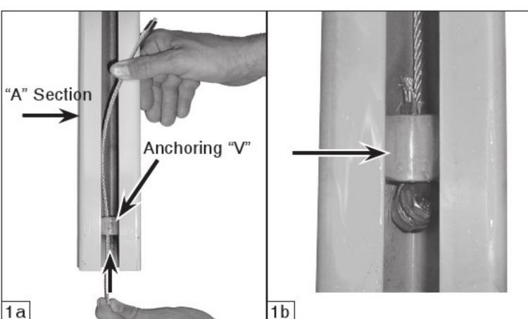
1a. Feed the crimped end of the new cable through the "A" section anchoring "V" from the bottom as shown. 1b. Make sure the anchoring end of the cable is pulled snugly against the anchoring "V" as shown. (NEVER DISASSEMBLE THE NUT AND BOLT OF CABLE ANCHORING ASSEMBLY)
