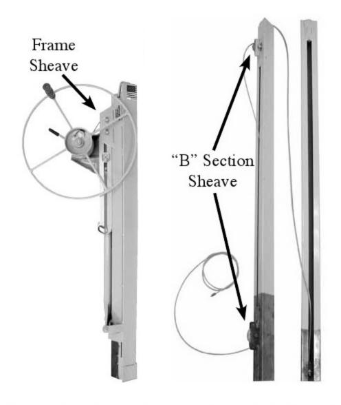
Inspect and replace sheaves (pulleys) before replacing the cable. There are 3 sheaves on the 138-2 Panellift\*, one on the frame and two on the "B" telescoping section.
