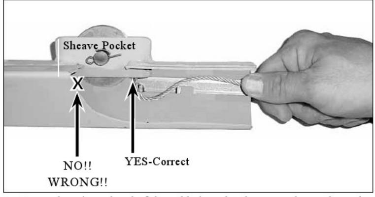
3a. Insert the crimped end of the cable into the sheave pocket at the end nearest the end of the "B" section as shown.
