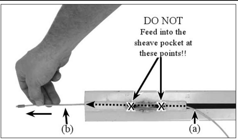
4. Feed the crimped end of the cable down into the slot (a) of the "B" section and out the bottom end of the telescoping section (b) as shown. Pull the cable completely through to remove the slack.
