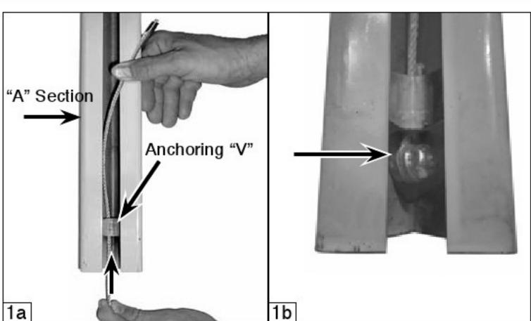
1a. Feed the crimped end of the new cable through the "A" section anchoring "V" from the bottom as shown. 1b. Make sure the anchoring end of the cable is pulled snugly against the anchoring "V" as shown.
