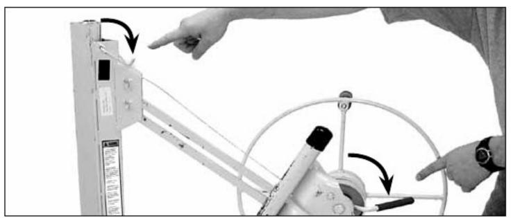
When the winch is fully extended, release the brake arm and swing the retaining hook away from the telescoping sections.
