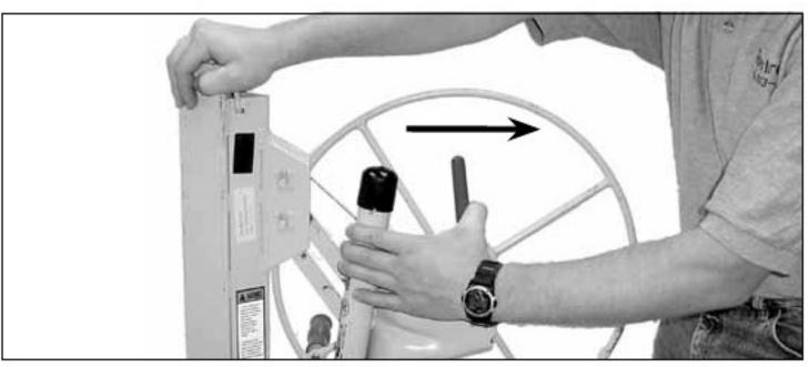
Place your right hand on top of the frame and pull the winch assembly towards you. While pulling the winch towards you, grip the brake arm sufficiently to prevent back-lash of the cable on the winch.
