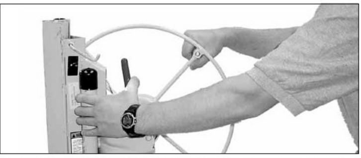
4. Raise the brake arm all the way up, grasp the winch post, and squeeze the brake arm firmly as shown.
