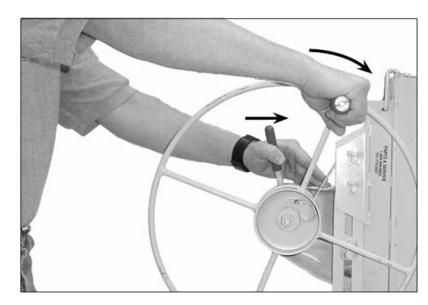
To move the winch into the working position rotate the winch forward slightly with your right hand while raising the brake arm with your left hand.
