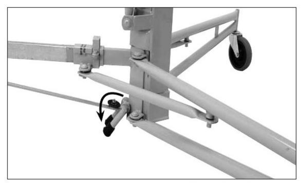
2c. To hold the tripod base in position during this procedure set the backstop as shown.
