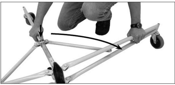
Begin by setting up the tripod base: press down on the slide yoke pin clip and swing the outer legs out until they lock in the working position (note the holes on the bottom of the slide tube).
