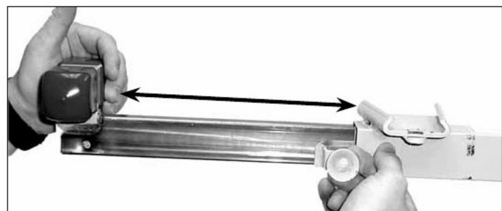
10. To extend the outriggers for use, pull out on the outrigger lock pin with your right hand and slide the outrigger out with your left hand as shown. The lock pin will engage at three different points on the outrigger: fully retracted, extended 21", or extended 33". MAKE SURE that the lock pins are engaged in one of these three positions before loading the unit. DO NOT use the PANELLIFT® with the outriggers extended beyond the 33" point.
