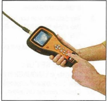
The status screen shows the capacity of the SD card and the internal battery. If the Micro-Scope has been stored for a long time the display might not have enough power to turn on. Please use the power adapter to re-charge the battery. Make sure you plug the power adapter into the port closest to the keypad on the command module.
