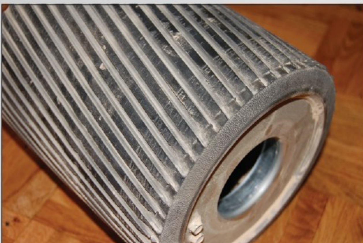
Pic. 7 Heavily used up drum ( 8 years old )
