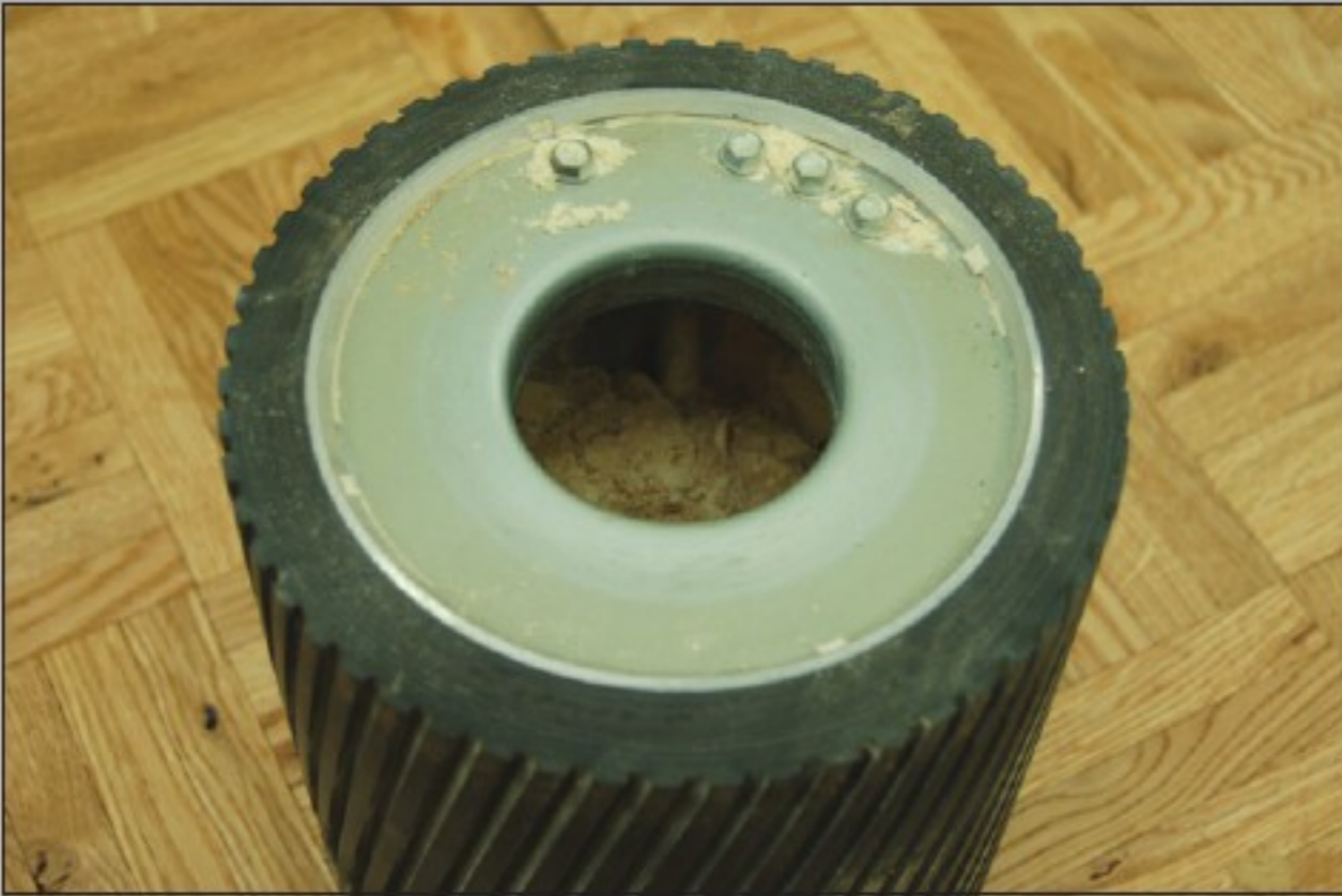
Pic. 9 Dust and debris in the drum
