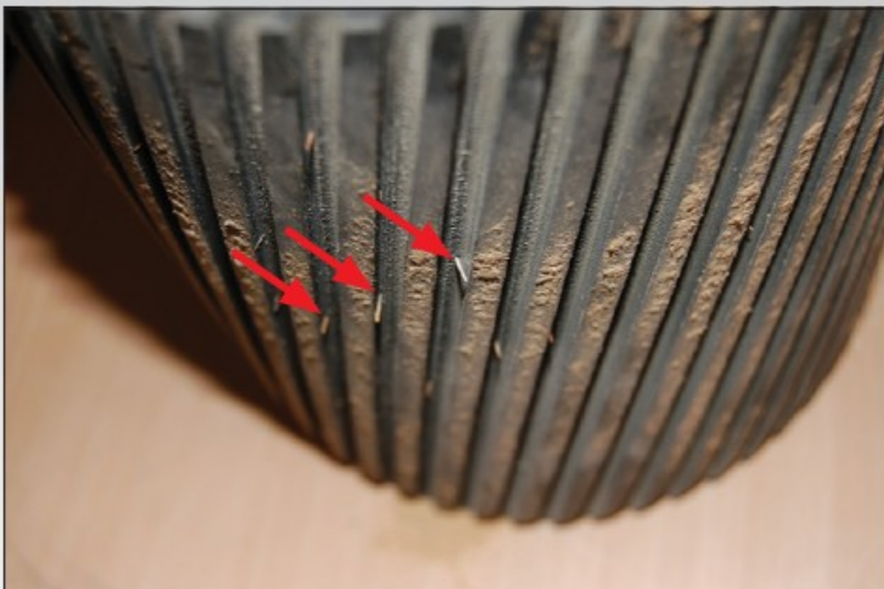
Pic. 3 Metal pieces in the rubber
