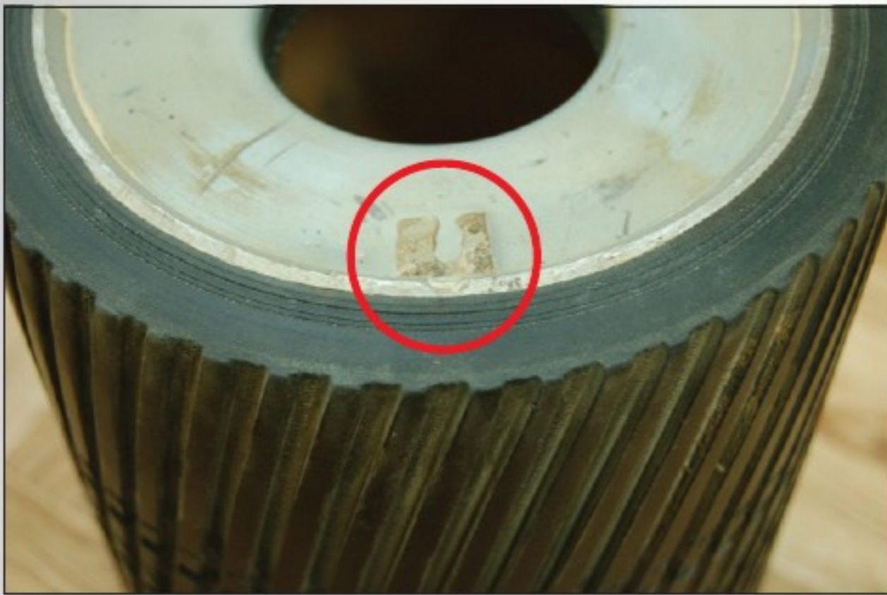
Pic. 5 Missing balancing weight
