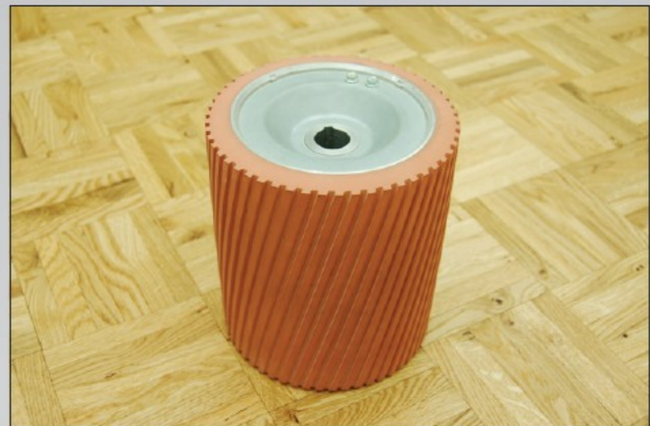
Pic. 12 Hard drum for softwood with lots of knots
