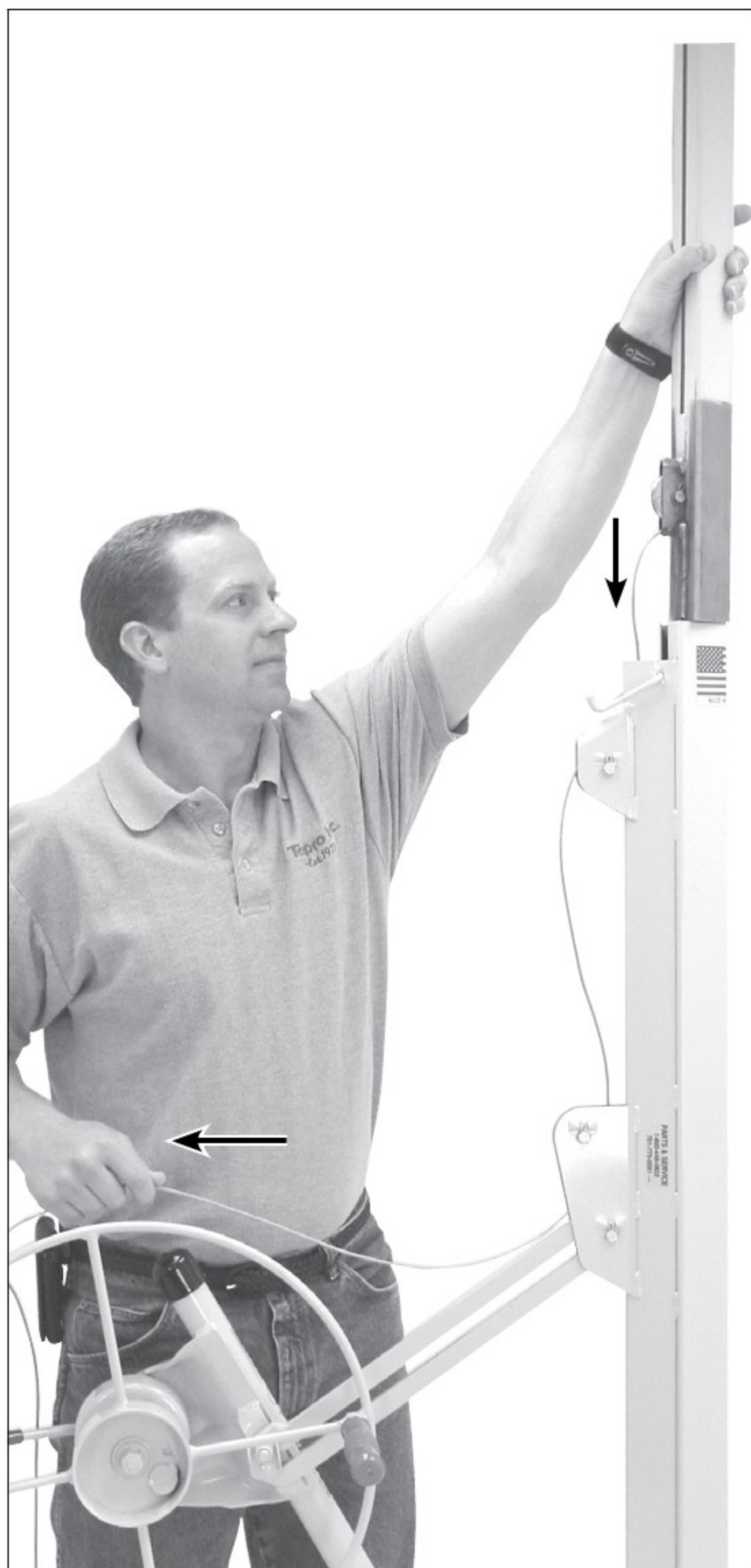
9. Pull the slack cable through the sheave pocket toward the winch and slide the telescoping sections into the frame housing. As the telescoping sections lower into the frame housing, the slack cable will be drawn back through the sheave pocket. Secure the cable correctly to the winch as shown in steps 9 - 10 on page 12
